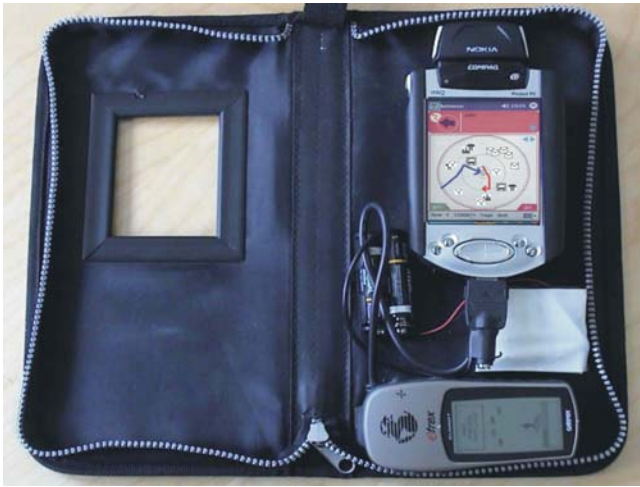
Figure 2. InfoRadar consists of a PDA supplemented with an electronic compass, GPS, GPRS receiver, a pen, and batteries packed to a nylon casing.
